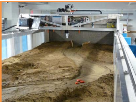
The instrument carriage maps a meandering stream created in the flume.
