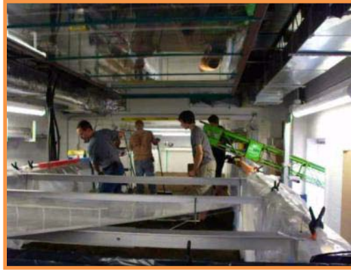
Manual labor spreading the sediment.
